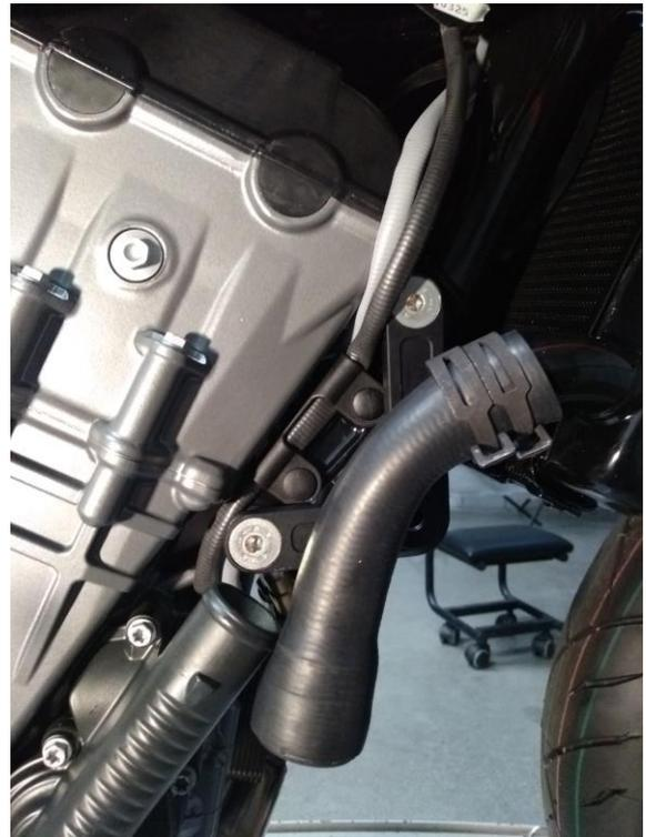
Install the protection as shown in the photo. Then re-install the sleeve.
